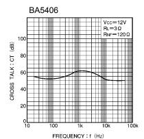
Fig.11Crosstalk vs frequency
