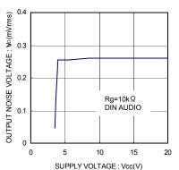
Fig.22 Output noise voltage vs Supply voltage
