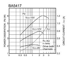
Fig.28 Power dissipation, circuit current vs. Supply Voltage( $RL=4\Omega$ )
