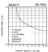
Fig.38 Starting time vs. Supply Voltage
