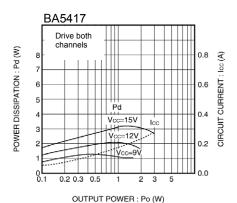
Fig.29 Power dissipation, circuit current vs. Supply Voltage (RL= $8\Omega$ )
