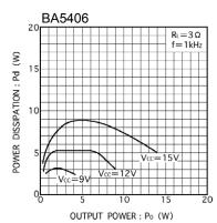
Fig. 17 Power dissipation vs Output power(3)
