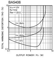
Fig.13 Distortion vs Output power
