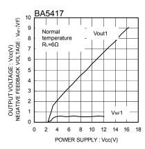
Fig.39 Output voltage, Negative feed back voltage vs. Supply Voltage
