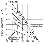
AMBIENT TEMPERATURE : Ta (℃) Fig.8 Thermal derating curve
