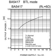
Fig.31 Rated output power vs. Supply Voltage
