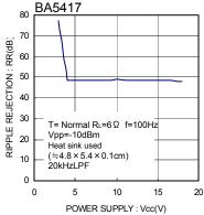
Fig.33 Ripple rejection ratio vs. Supply Voltage
