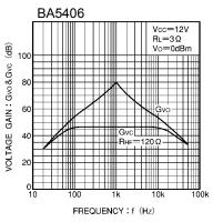
Fig.10 Voltage gain vs frequency
