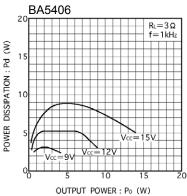
Fig.15 Power dissipation vs Output power(1)
