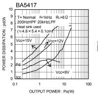
Fig.35 Power dissipation, Supply current vs. Frequency
