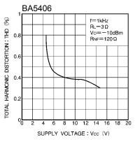
Fig.12 Distortion vs power supply voltage
