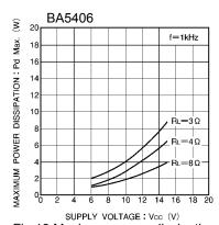
Fig.18 Maximum power dissipation vs Supply voltage
