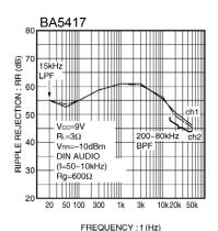
Fig.24 Ripple rejection vs. Frequency
