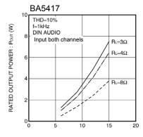
Fig.20 Rated output power vs Supply voltage
