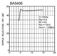
Fig. 19 Ripple rejection ratio vs Supply voltage
