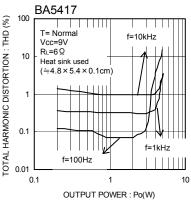
Fig.32 Total harmonic distortion vs. Output power
