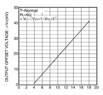
Fig.40 Output offset voltage vs. Supply Voltage
