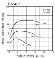
Fig.16 Power dissipation vs Output power(2)
