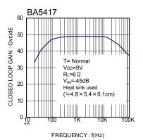
Fig.34 Close loop gain vs. Frequency
