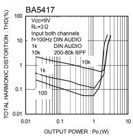
Fig.21 Total harmonic distortion vs Output power
